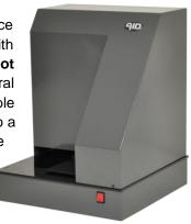
The **AID vSpot Spectrum** is equipped with an 8 position filter wheel, which allows for a customized selection of up to 7 individual narrow-band fluorescent filters, whilst still allowing for our "one-click switch" to perform enzymatic analysis via LED illumination on different plate formats.
